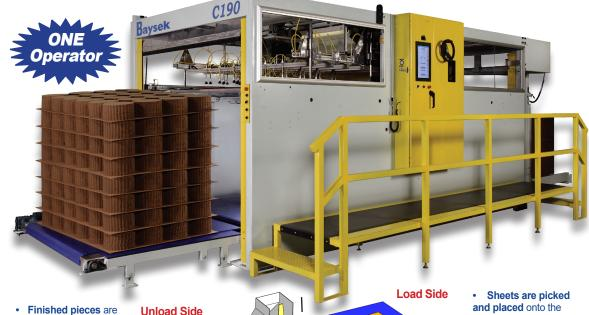
held in the die via suction cups while waste is automatically stripped up the waste hood and directed to recycling
