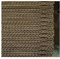
POWERFLUTE IS USED FOR ADDED STRENGTH AND MOISTURE RESISTANCE.
